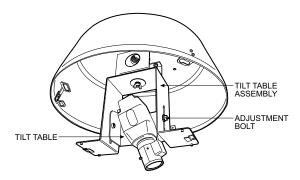
Figure 2. Camera and Lens Installation
